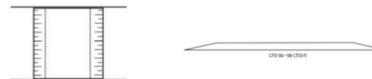
**Proposed - Watt's profile road hump** - Generally reduces traffic speeds by 45%
