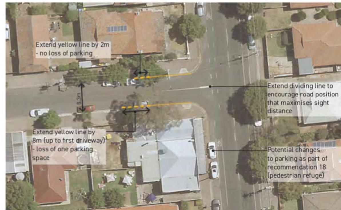
Figure 6.18 Recommendation No Stopping zone extension
